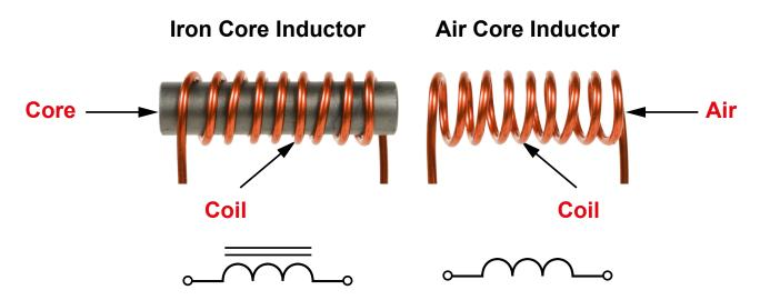
A current "i" flowing through the coil of an Inductor develops a voltage potential "e" across its contact leads and temporarily stores electric energy in a magnetic field within the core and around the coil. The core increases the inductance and efficiency of an **Inductor** by concentrating the magnetic flux lines of the field entirely within its closed magnetic path structure.
